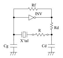
1) Connect the resister(R) to the circuit in series with the crystal unit.
