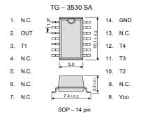
Function Connected to a positive power supply. OUTPUT 32.768 kHz clock output pin (C-MOS).
