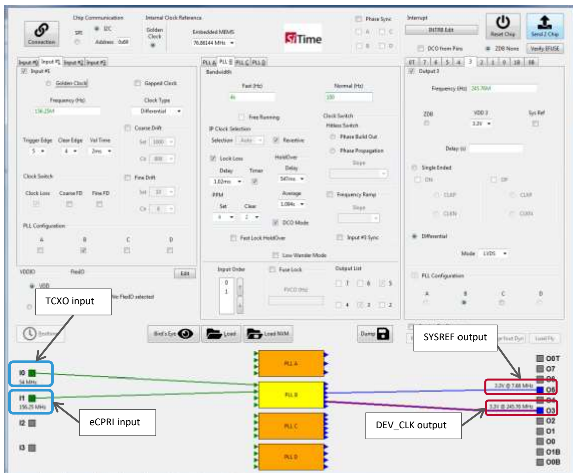
Figure 78: Example of the initial configuration of SiT95148 for JESD204B
