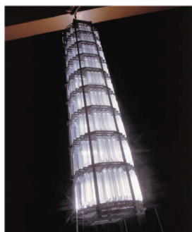
Artificial quartz crystal drawn from an autoclave
